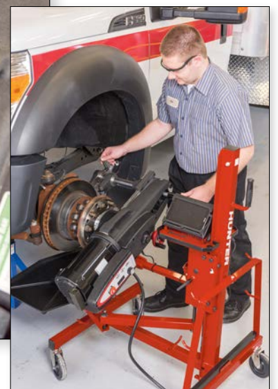
Optional accessories will give the capacity to service larger rotors found on medium-duty vehicles
